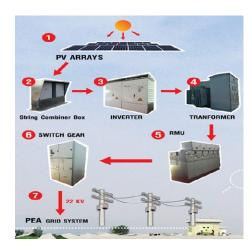
THE PICTURE OF THE PRODUCTION PROCESS OF ELECTRICITY FROM SOLAR ENERGY BY PV SYSTE
